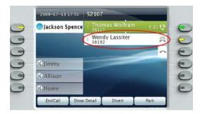
To connect the second call and put the first call on hold automatically, press the flashing amber session button (right side).
