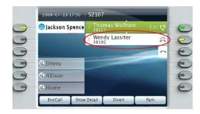
To connect the second call and put the first call on hold automatically, press the flashing amber session button (right side).
