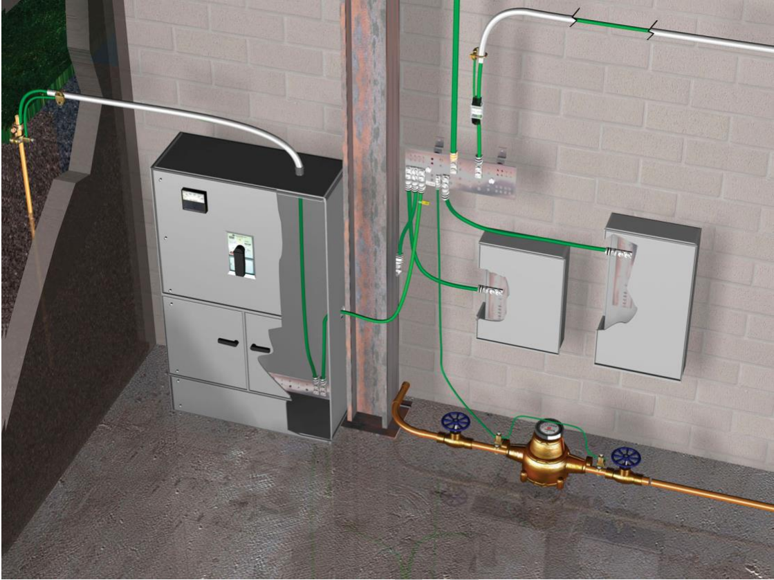
Figure 3: Grounding and Bonding at the Service Entrance
